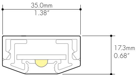
The LEDX-4 has been designed with corrugated side baffles which reduce direct view of the LEDs; the corrugations diffuse the effect of the hot spot.
